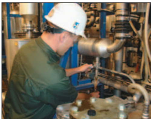
THE REAL McCoy: Jeff Knutson siphons off pure corn oil from an extraction process. It's currently used to make biodiesel, and could be the feedstock for food-grade corn oil, as well.
